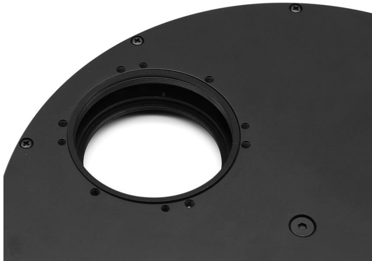
Figure 7-5 7x2" filter wheel, darkening gasket B used
