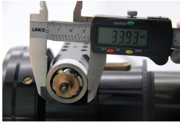
Figure 5-4 Measure the diameter for clamp
