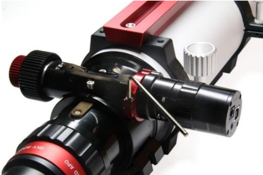
Figure 2-14 Tighten the clamp
