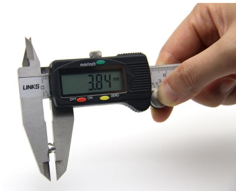
Figure 8 Measurement of a M4 screw
